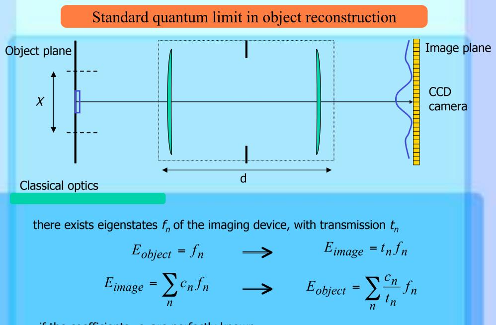
if the coefficients  $c_n$  are perfectly known, object shape can be reconstructed **without limitation due to diffraction**
