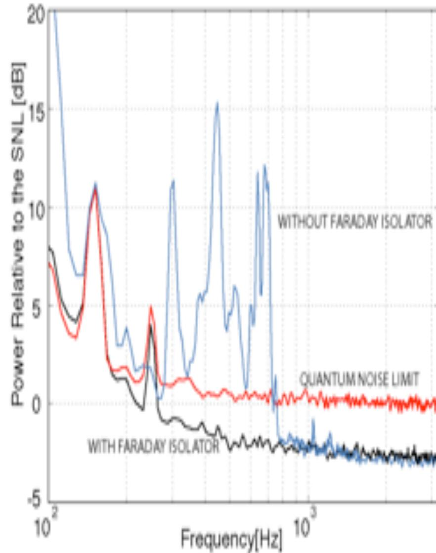
RBW = 8Hz, No.RMS ave = 400 without isolator, 500 for QNL and with Isolator. Electronic noise (not shown) was not subtracted
