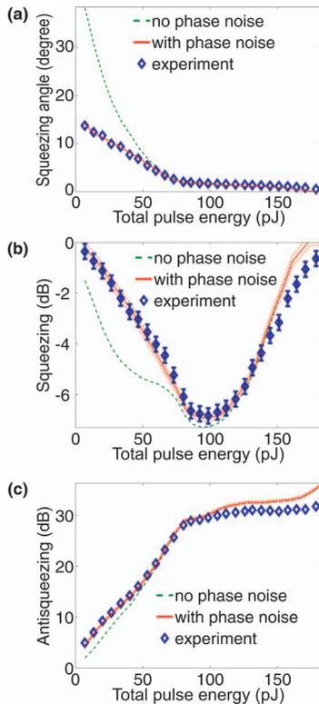
Fig. 3. Diamonds show the experimental results of the (a) squeezing angle, (b) squeezing, and (c) antisqueezing for the 13.2 m fiber. Error bars on the squeezing data indicate the uncertainty in the noise measurement; for the antisqueezing, the error bars were too small to be plotted. Solid and dashed curves show the simulation results with and without additional phase noise, respectively. Dotted curves indicate the sampling error in the simulation results.
