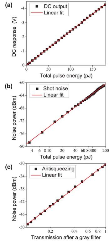
Fig. 2. (Color online) Plots of (a) dc response of one of the detectors pair, and (b) noise power measured at 17.5 MHz by the minus output of the detectors pair versus the optical pulse energy from the fiber. (c) Measured antisqueezed noise as a function of the transmittance after a gray filter.
