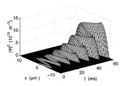
FIG. 3. Growth of a BEC with a center-of-mass oscillation present. Shown is the condensate density  $|\Psi(x,t)|^2$ , as found from the asymptotic solution in a symmetric trap, with a center-of-mass oscillation in the x direction and N(0) = 10. The gain coefficient is chosen as  $g = 0.1\omega$ , while  $a_{0,1} = 4.86 \mu \text{m}$  and  $\delta_{0,1} = \pi/2$ . Other parameter values are as previously.
