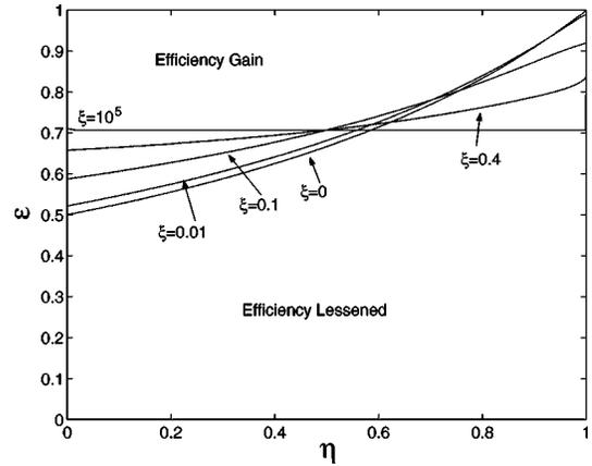
FIG. 4. Regions of efficiency gain for the single-copier ( $N=1$ ) detection scheme, as a function of  $\varepsilon$ , the copier, and  $\eta$ , the detector efficiencies, for varying frequency of dark counts parametrized by  $\xi$ . In all cases, the copier produces vacuum when it fails ( $\mu=-1$ ) and the input is equiprobable to be a photon or vacuum ( $p=1/2$ ).
