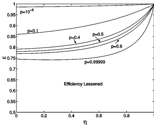
FIG. 6. Regions of efficiency gain for the single-copier ( $N = 1$ ) detection scheme, as a function of  $\varepsilon$ , the copier, and  $\eta$ , the detector efficiencies, for varying *a priori* photon input probabilities  $p$ . In all cases, the probability of dark counts in the detectors is taken to be zero ( $\xi = 0$ ), and the default output upon copy failure is a totally random state ( $\mu = 0$ ). Note that the scale in  $\varepsilon$  differs from that in Figs. 2, 4, and 5.
