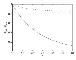
FIG. 1. Minimum state preparation fidelity  $\epsilon_{\min}$  for ideal detectors (solid line), and minimum detection efficiency  $\eta_{\min}$  for ideal state preparation (dashed line) required for violation of (8) as a function of the number of modes. The asymptotic value of  $\eta_{\min}$  is indicated by the dash-dotted line.
