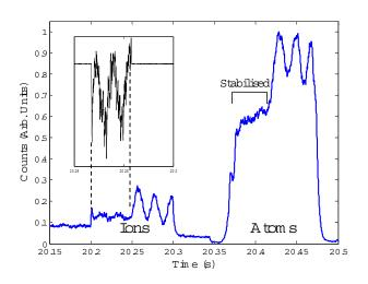
Fig. 1: Electron multiplier trace, averaged over four runs of the experiment, demonstrating stabilisation of the atom laser beam. The ion signal is first to arrive on the left of the trace, while the atom signal arrives  $\sim$  150 ms later which is the time of flight from the BEC to the EM. Shown in the inset is the output of our control circuitry.
