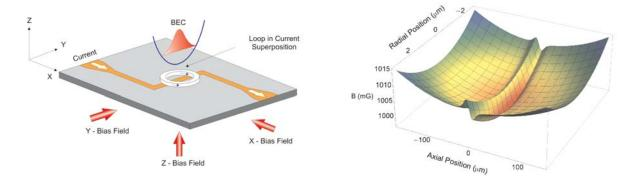
Fig. 1: Schematic of an atom chip containing the superconducting loop.
