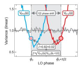
Fig. 1: Results for inseparability. Measurement of the variance for the sum  $V_{x'+y'}(\phi)$  and difference  $V_{x'-y'}(\phi)$  for the 45° rotated fields. The data, both below the QNL, are combined to one value for the inseparability of  $\mathcal{I} = 0.82 \pm 0.02$ , demonstrating significant entanglement between two orthogonal spatial modes within one optical beam.
