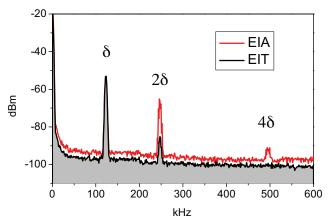
Fig. 1: Four-wave mixing spectra obtained for drive and probe fields separated by  $\delta \simeq 125 \text{ kHz}$ .
