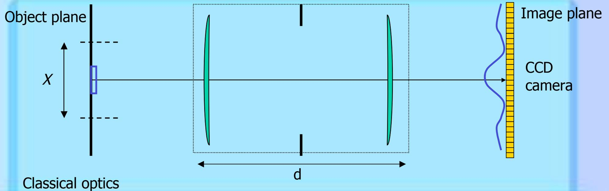
there exists eigenstates  $f_n$  of the imaging device, with transmission  $t_n$
