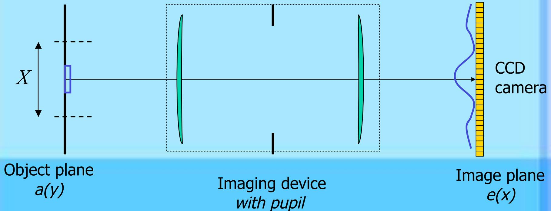
There exist **eigenmodes of the system** (*prolate spheroidal functions*),  $f_k(x)$  with eigenvalues  $t_k$  (transmission coefficient).
