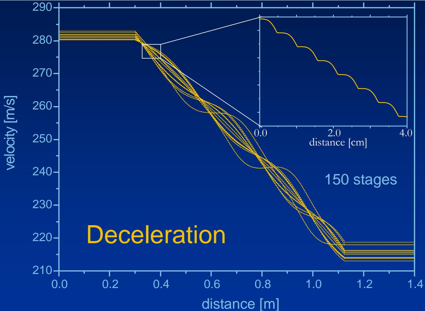
$v_{\text{start}} = 282 \text{ m/s}$ , distance of stages 5.5 mm
