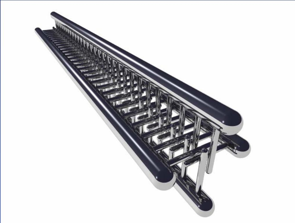
The first decelerator will have 100 stages and should reduce the velocity from 285 m/s to 240 m/s.
