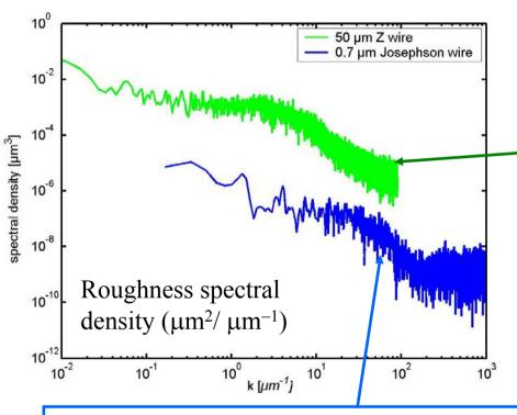
Orsay 1<sup>rst</sup> generation: electroplated gold wires (5 µm x 50 µm) on silicon wafer:
