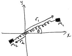
As the system is rotating around the centre of mass, we know  $m_1r_1 = m_2r_2$ , i.e.  $r_2 = \frac{m_1}{m_2}r_1$ . Then
