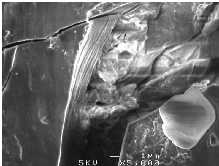
Figure 8.3: Scanning electron micrograph of a pressed pellet of melanin powder. Sample not coated in platinum. Magnification is 5K. Image taken by Shuzhi Cai.
